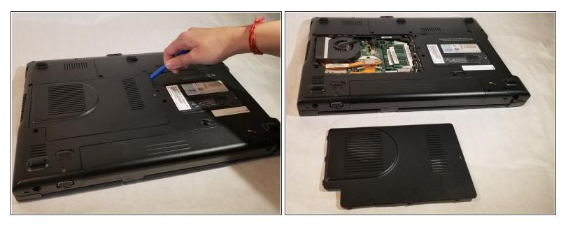
Insert the plastic prying tool and pry the back panel off starting at an edge and moving your way around it.
