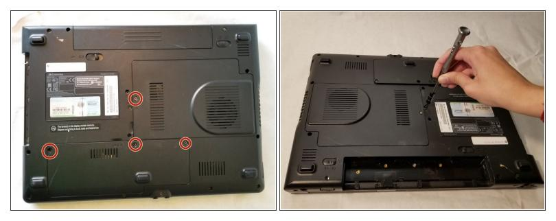
• Using the Phillips #1 screwdriver, remove the four 6mm screws on the back of the laptop.
