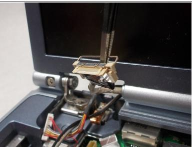
Use tweezers to grab onto the lever to remove the chip from the motherboard.
