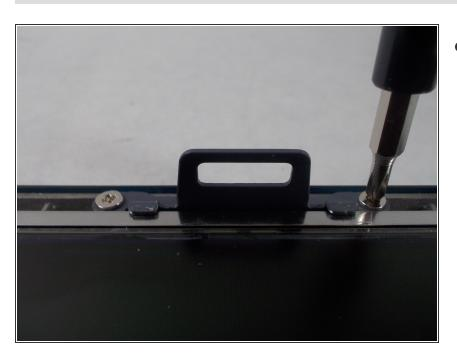
Remove the 3mm screws with a Philips head #00
