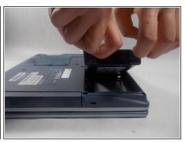
↑ To prevent injury, make sure the laptop is unplugged and turned off before removing the battery.
