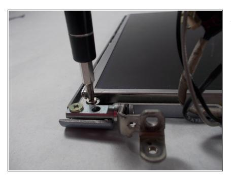
Remove the 2.5mm screws with a Philips head #0 on both sides of the laptop
