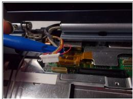
Use a plastic opening tool to lift up both sides of the white tab.
