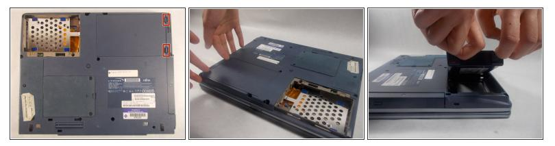
To prevent injury, make sure the laptop is unplugged and turned off before removing the battery.
