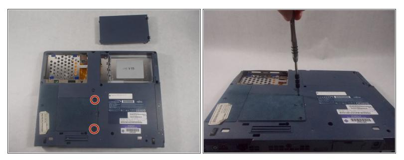
Use a Philips head #0 to remove the 4mm screws to the RAM cover.
