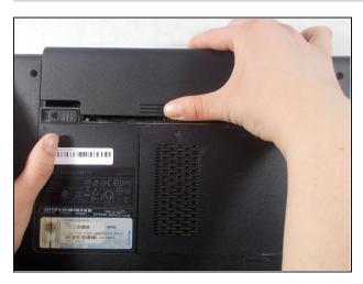
Push upward from the base of the battery.
