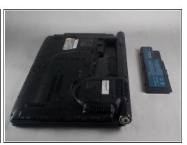
Pull the battery up and out. Use a plastic opening tool if necessary.
