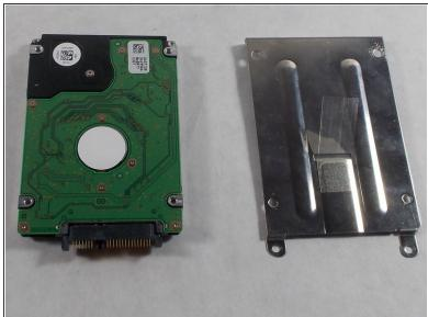
Lift the casing off the hard drive.
