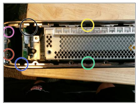
• To take off the frame, take a flat head screwdriver and pull of the latches until it comes off.
