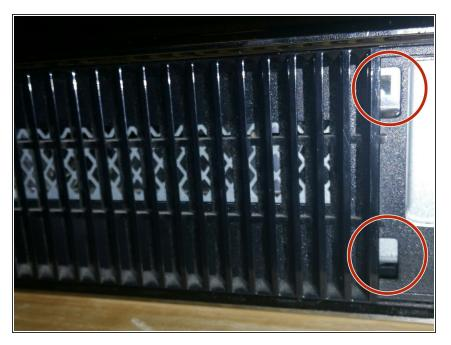
Take a flat head screwdriver and pull up on the two ends of the side cover.
