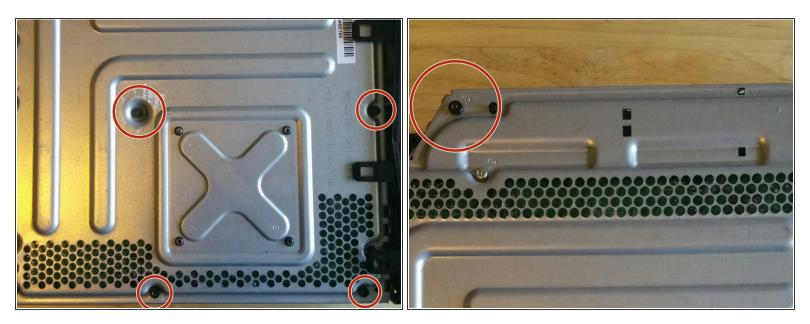
Use your T8 and T10 Torque screwdriver and take out the five black screws that are shown in the picture.
