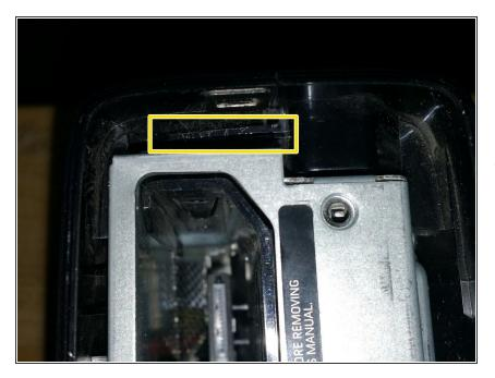
On the other side, take your flat head screwdriver and unlatch the latch. There is a harder latch farther inside so you have to stick the screwdriver far down and try to find it by feeling around. It helps to push both sides of your Xbox security sticker.
