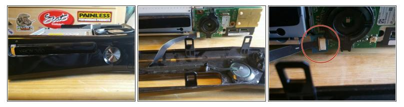
• Take your front cover with your home and eject button and lay it down in front of the console. The front cover is connected to a power source by the home button. Be very careful to pull it over and then out so you don't break it.
