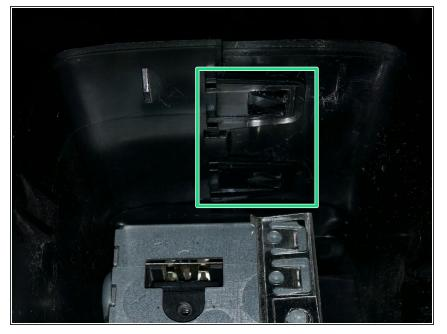
• Take your flat head screwdriver and unlatch the two latches and then place a different screwdriver through the latch so it doesn't latch.
