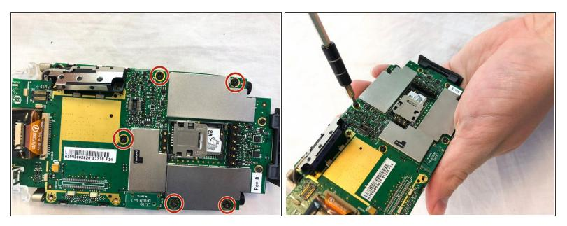
• Remove the five 3mm Phillips #00 screws from the motherboard.
