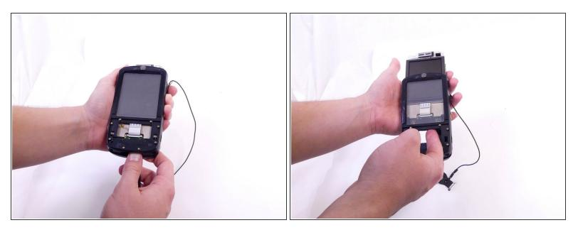
• Using your finger, or spudger, push the motherboard out from the bottom.
