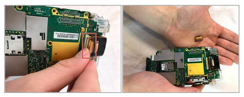
Remove the scanner ribbon cable by pulling straight up and out.
