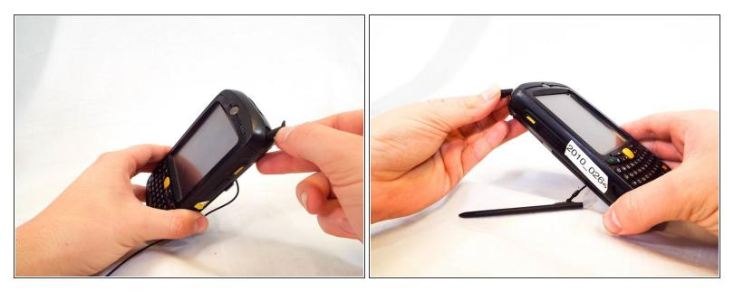
• Remove the two rubber plugs on the top of the device by pushing them up and out of the phone.
