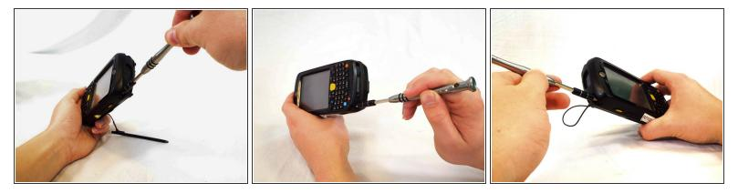
• Remove the four 1cm Phillips #0 screws from the top and bottom of the phone.
