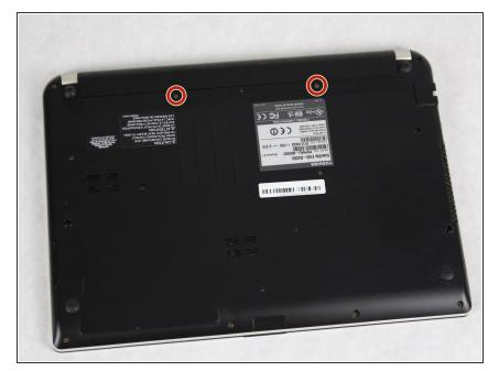
Remove the two 4 mm screws securing the battery on the back side of the laptop with a Phillips #1 screwdriver.
