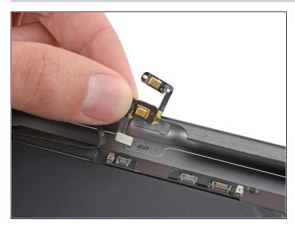
• Remove the dual microphone assembly from the iPad.
