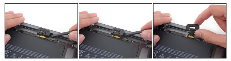
Use a spudger to pry the front-facing camera housing up and lift it out of the case.
