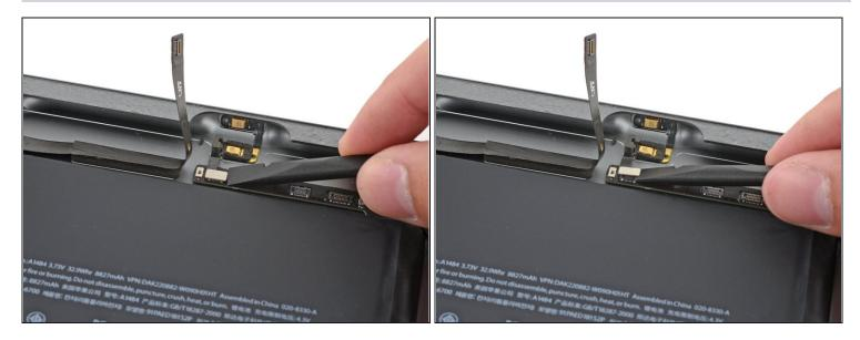
• Use the flat end of a spudger to disconnect the microphone cable connector from the logic board.
