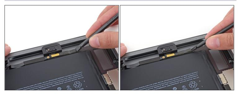
• Use the flat end of a spudger to disconnect the front-facing camera connector from the logic board.
