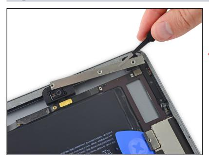
• Remove the upper component cable bracket.
