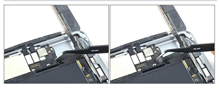
• Remove any tape covering the home button ribbon cable connector.
