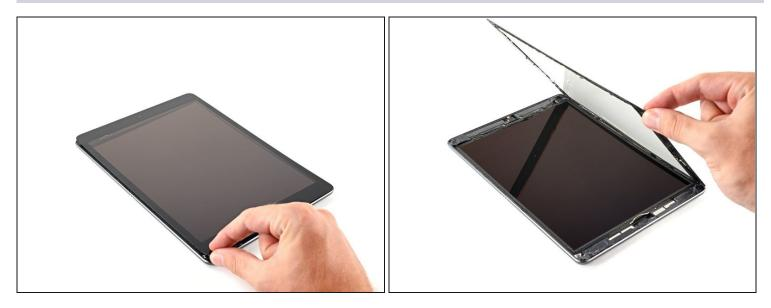
• Lift the left edge of the digitizer upwards to further separate the adhesive along the right edge of the iPad.
