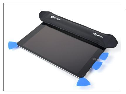
• Heat an iOpener and apply it to the right edge of the device for two minutes.
