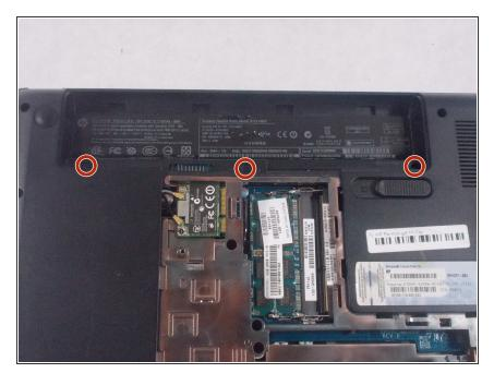
Remove 3 screws located where the battery previously was.
