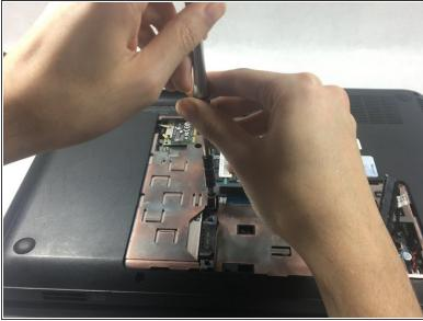
• Remove 6 screws located under the spot where the smaller L-shaped panel was located.
