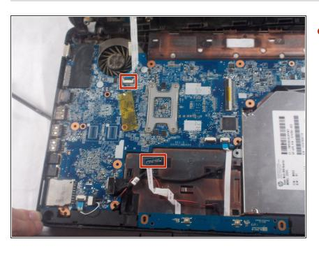
Unplug wires connecting back panel to keyboard.
