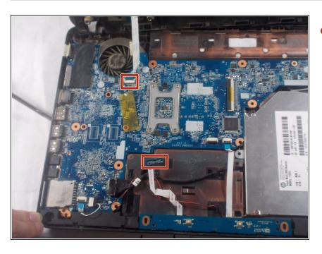
Unplug wires connecting back panel to keyboard.
