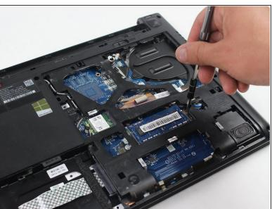
Remove the nine 7mm screws with a JIS #0 screwdriver.
