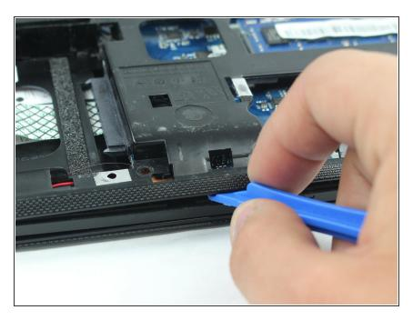
Using the plastic opening tool split open the laptop on the ends.
