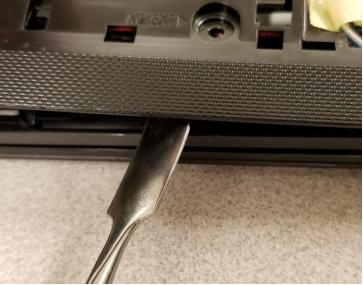
• Use a spudger at the edges of the laptop cover to carefully pry upwards, removing the cover.
