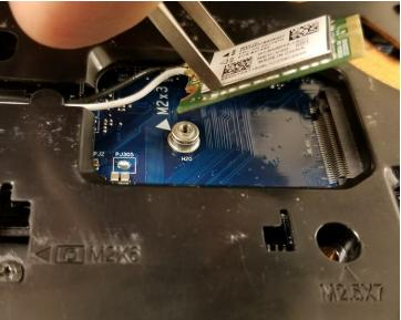
• Remove the 3mm screw and carefully pull out the cables from the hooks holding them in place.
