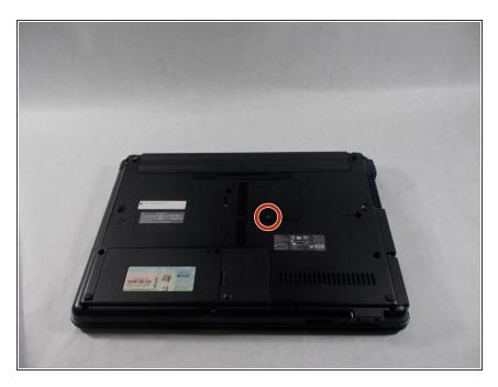
Turn the laptop over. The screw for the RAM is located in the middle of the device.
