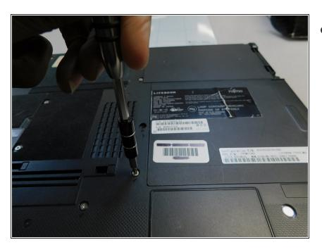
Remove the two Phillips #0 screws from securing the optical drive.
