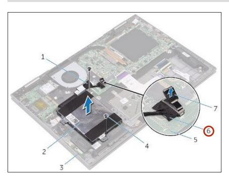
Using the pull tab, disconnect the hard-drive cable from the system board.
