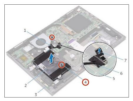
Remove the two screws (M2x3.5) that secure the hard-drive assembly to the palm-rest assembly.
