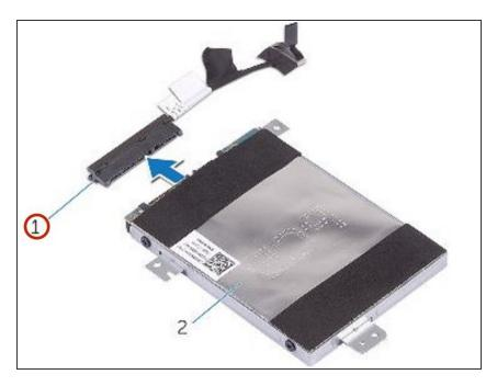
Disconnect the interposer from the hard-drive assembly.
