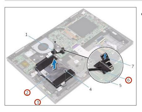
Lift the hard-drive assembly, along with its cable, off the palm-rest assembly.
