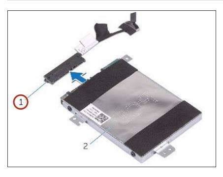
Connect the interposer to the harddrive assembly.
