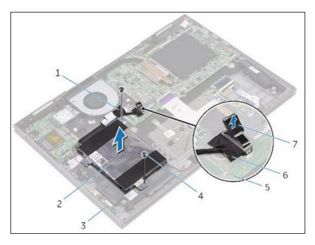
Replace the two screws (M2x3.5) that secure the hard-drive assembly to the palm-rest assembly.
