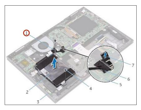
Adhere the tape that secures the hard-drive cable to the palm-rest assembly.
