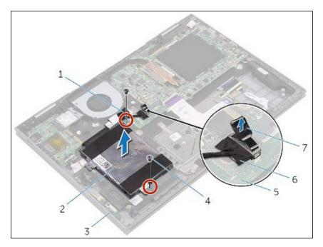
Align the screw holes on the harddrive assembly with the screw holes on the palm-rest assembly.
