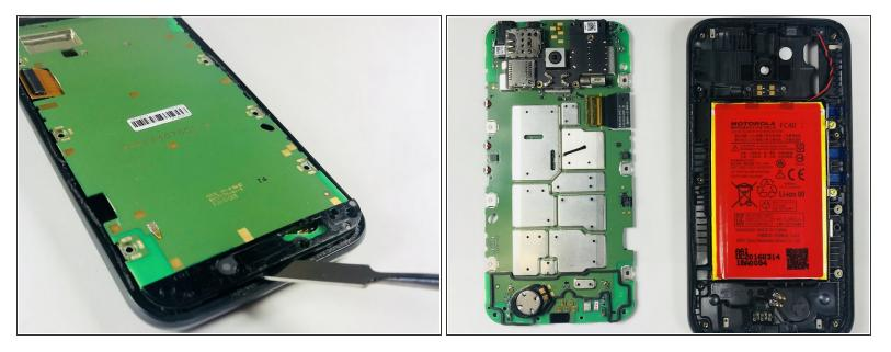
• Use the metal spudger and lift the back cover on the bottom side of the phone (this is attached to the motherboard).
