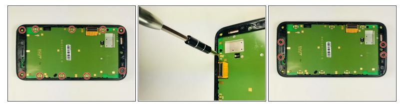
With a T4 screwdriver, remove the 10 "yellow" 2mm screws and 4 "black" 2mm screws.
