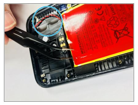
• Remove the red and black battery cable from its port using tweezers.
