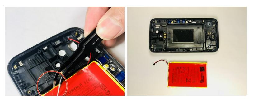
Use the same tweezers to remove the red battery from where it is placed.
