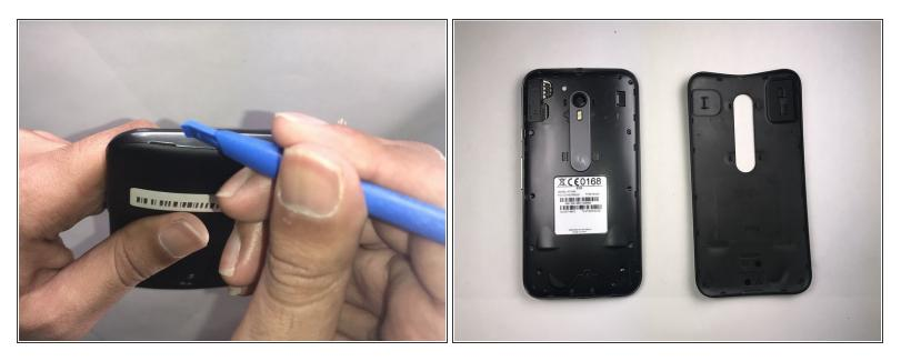
• Use the plastic opening tool to open the back cover as shown in the photo.
