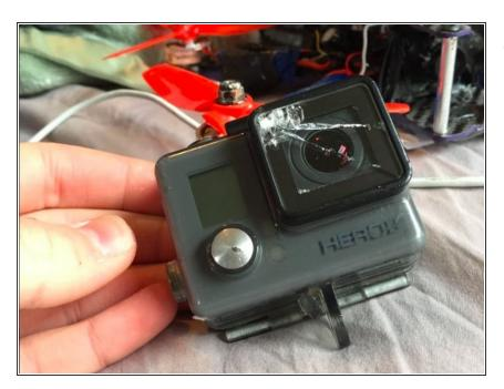
Cracked an irreplaceable glass lens cover, but all hope is not lost
