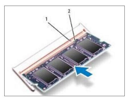
Align the tabs on the memory module cover with the slots on the computer base and snap the cover into place.
