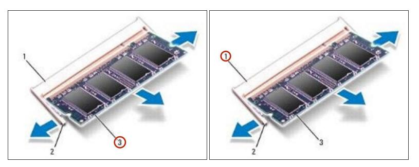
• Remove the memory module from the memory module connector.
