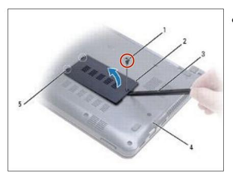
Replace the screw that secures the memory module cover to the computer base.
