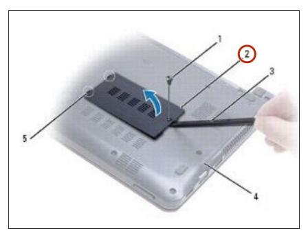
• Use a plastic scribe to lift the memory module cover up at an angle and ease the tabs out of the computer base.
