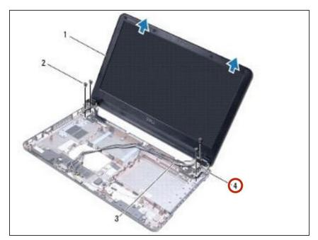
Slide the hinges out of the slots in the computer base.
