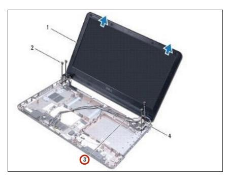
Route the Mini-Card antenna cables through the routing guides on the computer base.
