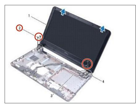
Replace the four screws that secure the display assembly to the computer base.
