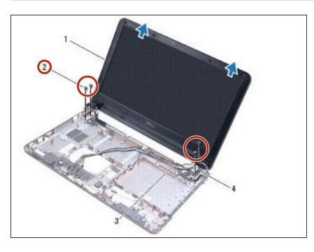
Remove the four screws that secure the display assembly to the computer base.
