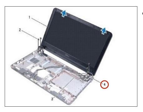
Slide the tabs on the display hinges into the slots in the computer base.
