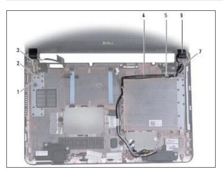
Align the display assembly with the computer base using the alignment posts on the computer base and set the display assembly in place.
