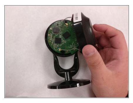
Remove the back casing to expose the circuit board.
