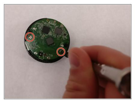
Remove the two 4.35 mm screws on the circuit board using the Philips head PH00 screw driver.
