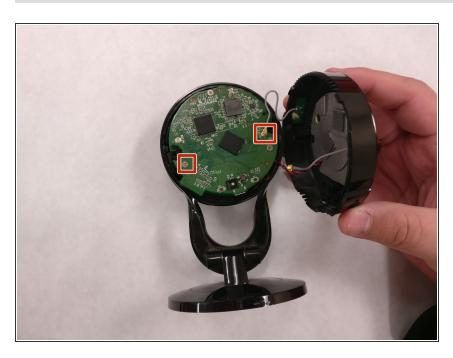
Detach the gray antenna wires by gently pulling on the side closest to the circuit board.
