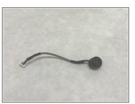
• Detach the microphone from the circuit board by gently pulling on the grey wire.
