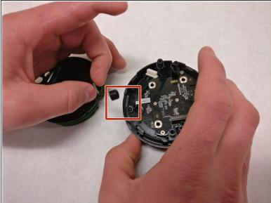
Gently pull on the grey wire to detach the microphone from the camera body.
