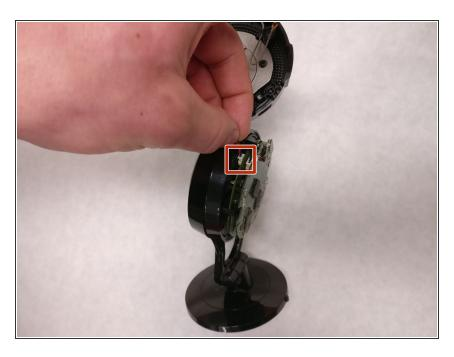
Detach the speaker wire by gently pulling on the side closest to the body of the camera.
