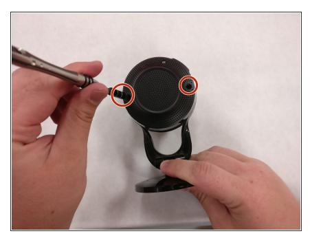
Remove the two 9.65 mm screws on the back cover using the Philips head PH00 screw driver.
