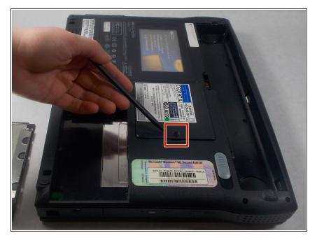
Locate the RAM on the bottom side of the laptop, the cover is secured by a 6 millimeter screw. Remove this with a Philips #1 screwdriver.
