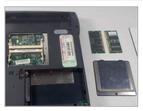
The RAM should be easily removed once released from the plastic clips.
