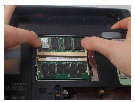
Place your thumbs on two of the clips securing one board. Push outwards on the clips. This should pop the board up.
