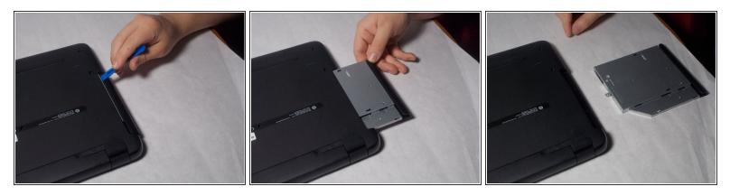
• Remove the disk tray assembly by sliding it out from the side using the blue plastic opening tool.
