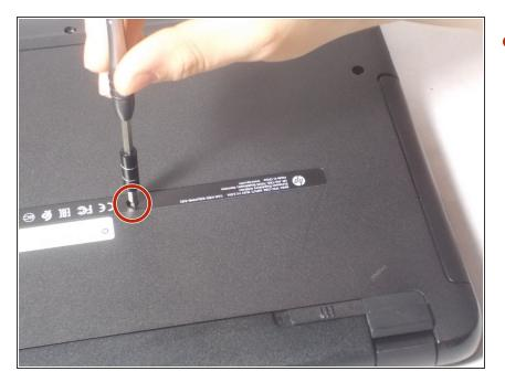
Using the Phillips #0 screwdriver, remove the 7.5mm screw from the underside of the plastic frame that holds the disc tray in place.
