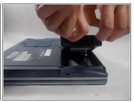
↑ To prevent injury, make sure the laptop is unplugged and turned off before removing the battery.
