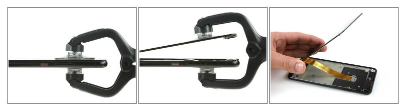
There is a thin display cable between the screen and phone, be very careful not to rip it when opening the device.
