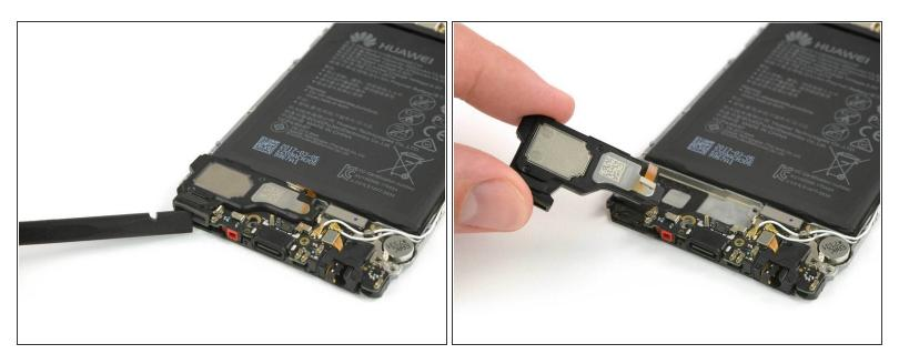
$\bigwedge$  Only insert the spudger as deep as 1/16 of an inch to avoid damage.
