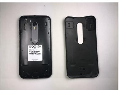
Use the plastic opening tool to open the back cover as shown in the photo.
