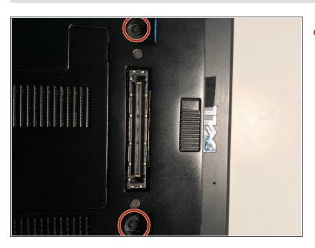
Flip the laptop over and remove the two Phillips #0 screws.
