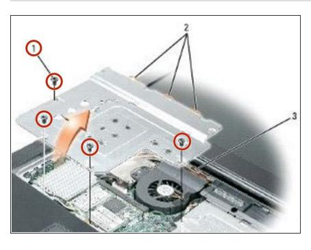
Remove the four M2.5 x 5-mm screws (labeled "M2.5x5") that secure the EMI shield to the system board.
