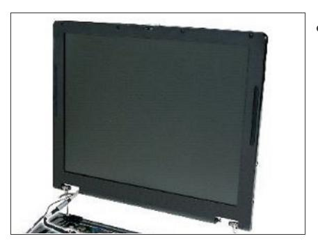
Lift the display assembly out of the computer base.
