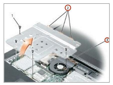
Pull the EMI shield out of the computer baseby rotating the front upwards then lifting to release the retention tabs from the retention-tab slots.
