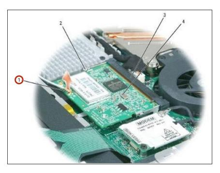
Disconnect the attached antenna cable from the Mini PCI card.
