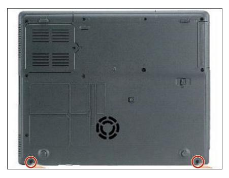
From the back of the computer, remove the two M2.5 x 8-mm screws labeled "D."
