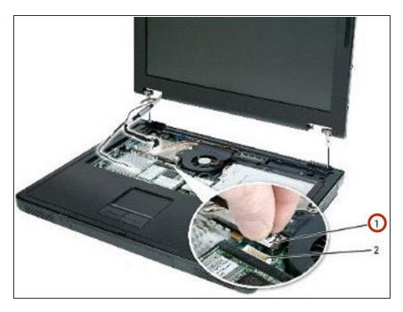
Carefully remove the Mini PCI card antenna cable and the display cables from their routing guides.
