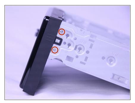
Remove the four 3.5mm Phillips #0 screws from the sides of the display.
