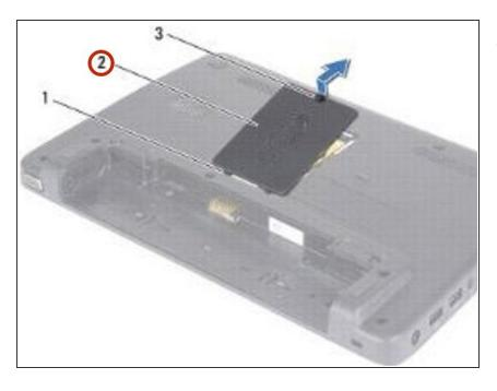
Lift the memory-module cover off the computer base.
