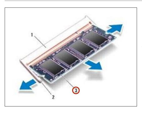
Slide the memory module firmly into the memory-module connector at a 45-degree angle, and press the memory module down until it clicks into place. If you do not hear the click, remove the memory module and reinstall it.
