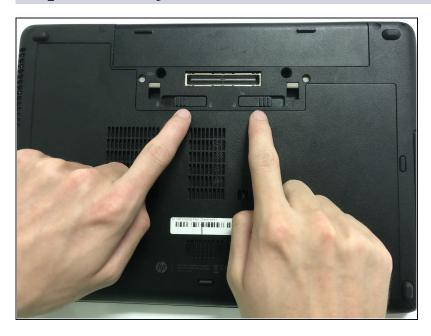
Locate the two slots on the bottom of the laptop to unlock the battery.
