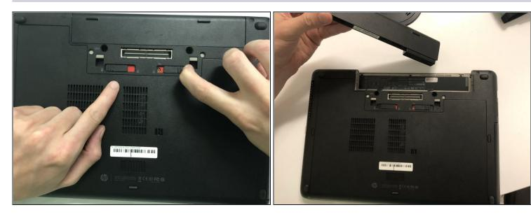
• Pull on both slots outwards as shown in the images to unlock the battery. The battery will not come out if the slots are locked. The battery should easily slide out without much force.
