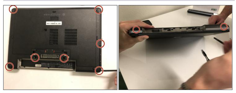
• Remove the nine screws that keep the back cover secured using the T5 Torx screwdriver.
