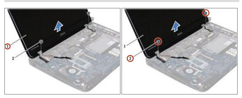
Place the NEW display assembly in position and replace the two screws (one on each side) that secure the display assembly to the computer base.
