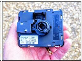
• Tip the centre console upside down and locate the ISM ignition switch. There are four spring clips holding it in place. Use a screwdriver to compress each clip in turn, whilst pushing the switch out of its socket.
