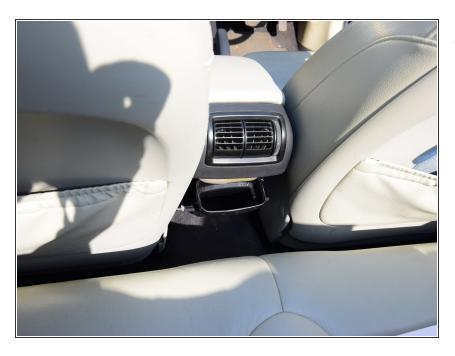
Underneath the air vent controlling air flow to the passengers from the center console sits a square duct.
