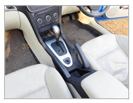
With all side panels in place, re-fit the screws around the gear lever and CD holder. Finally, slide the handbrake cover in place, and screw the CD holder in. All rubber mats put in place (you \*did\* clean them whilst you had the chance, right..?). You are done!
