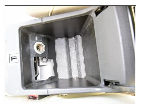
Remove the bottom rubber cover in the centre console storage unit.
