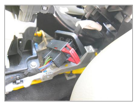
Push a screwdriver inside the red tab and pull, and the connector splits neatly apart.
