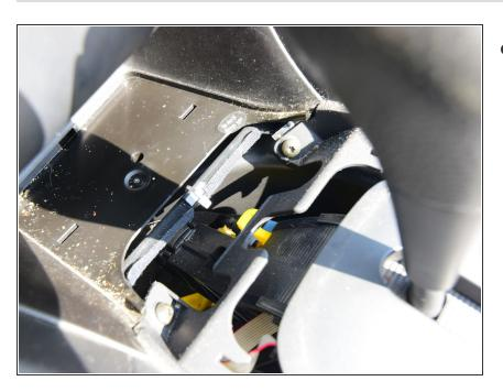
Remove two screws located in front of the gear lever.
