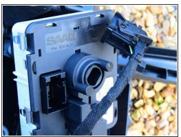
• The switch is connected to a cable via a connector. Locate the torque lever and twist this to release the connector.
