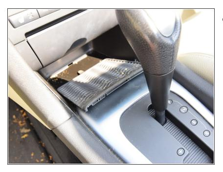
Next, remove the rubber mat in front of the gear lever.
