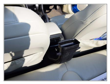
The Haynes manual suggests pulling this out next, and although it is possible to do so, it requires force, and is much easier to do later when all other fixings have been removed.
