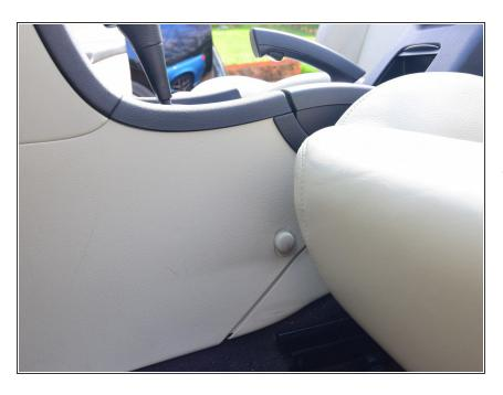
Step one is to remove the front side panels. There is a single (covered) screw in the footwell on each side
