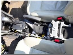
The center console is now loose, and can be puller backwards and upwards, and removed from the car.
