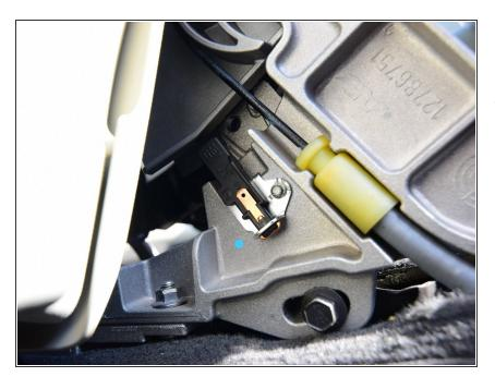
The other is an earth connector near the rear of the console. This can easily be pulled away.
