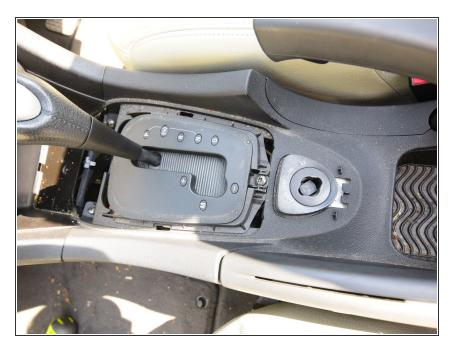
Removing the gear lever surround trim exposes a single screw holding a retaining frame underneath the gear change mechanism.
