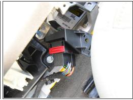
Connect the two cables. The earth connector is push-on, and the square plug self-locks when the red tab is pushed.
