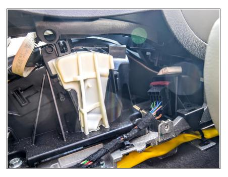
There are two cable bundles connected to the center console from the rest of the car. One is
