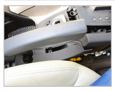
Slide out horizontally the protective plastic cover underneath the hand brake.
