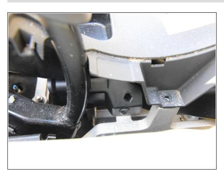
The next bit is a bit fiddly to get to: There are two screws going horizontally, one underneath the handbrake,
