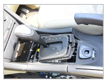
Remove the retaining frame
