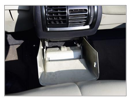
Next, locate the rear cover visible from the back seats, between the two front seats. Pull it sharply to the rear, and remove.
