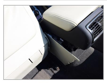
The rear side panels in front of the rear cover are now easily accessible and can be removed.
