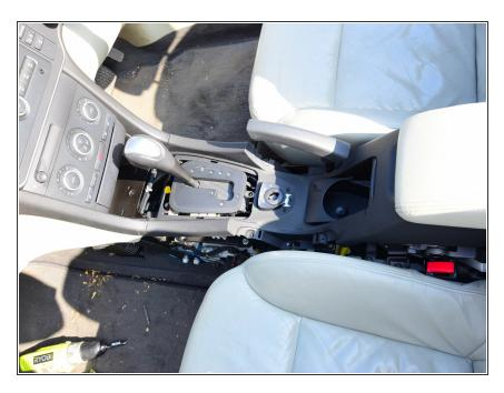
The square air conditioning duct goes in first. The console goes in next. It is a bit awkward to riggle past all the lugs, screws, tabs and cables, but just persevere. Once in, fit all the screws holding it in place, including the awkward ones.
