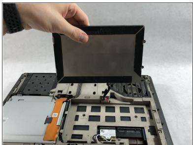
Pull battery up using the tab provided.
