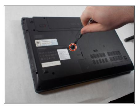
Remove the 9mm Phillips #0 screw holding the CD drive in place.
