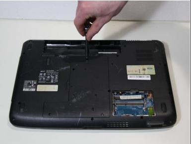
Unscrew the 2 captive screws and 3 M2.5 x L8 screws holding back cover in place.
