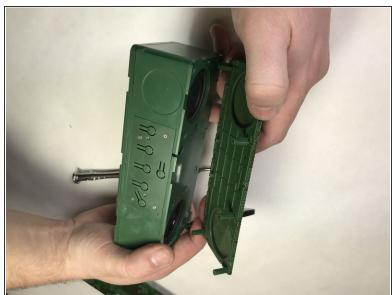
Lift the front plastic shielding from the device.
