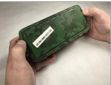
Run your hand around the device where the sleeve connects, lifting lightly up until the edges detach from the device case.
