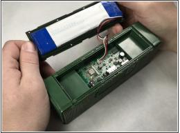
Using your hands, pry the panel off of the top of the device to reveal the device circuit board and the battery attached to the inner side of the panel.
