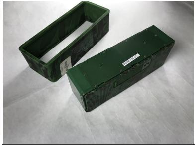
Turn the device around and gently push the speaker through until it separates from the sleeve.
