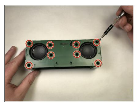
Using a Phillips #1 screwdriver, remove the eight 10mm screws on the revealed front panel.
