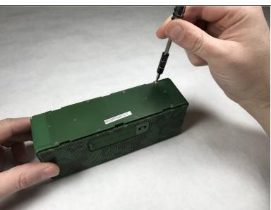
• Using a Phillips #0 screwdriver, remove the ten 5.1mm screws that hold down the battery panel on the bottom of the speaker unit.
