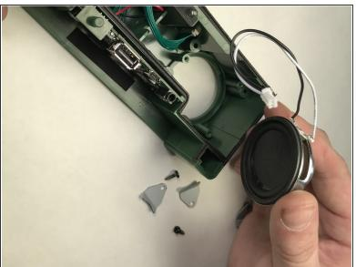
Using tweezers, detach the cord connecting the speaker to the device and lift out the speaker.
