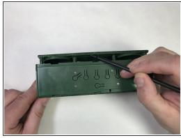
Using hands or a spudger, pry the front side of the plastic shielding (side opposite of power, control, and auxiliary port cover) from the device.
