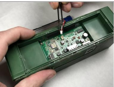
Using tweezers, carefully detach the battery wire from the circuit board and lift out the panel with the attached battery.
