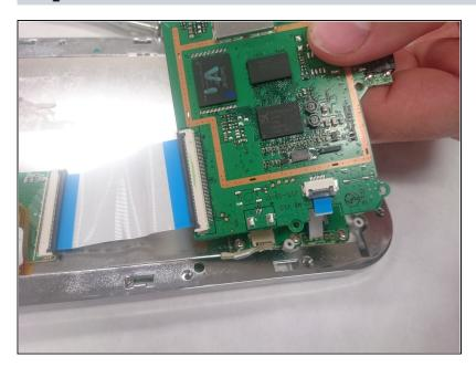
• Remove the circuit board.
