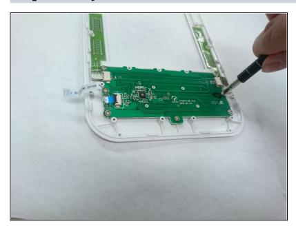
Remove the 10 Phillips head 4.2 mm screws using PH#00 screwdriver from the key board chip.
