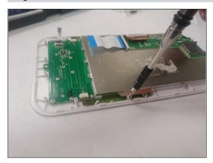
Remove screws from the large metal shielding.
