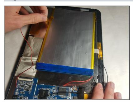
Remove the yellow tape holding the battery to the device using your fingers or plastic opening tool if necessary.
