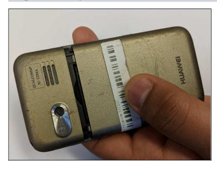
Depress the top of the battery cover, and pull downwards towards the base of the phone.
