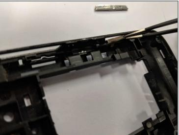
• Use a pair of <u>tweezers</u> to grab hold of each button on an edge from inside of the casing and pull out to remove.
