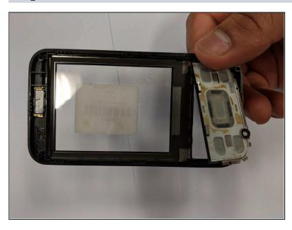
If it is the actual main screen panel control buttons that need to be replaced, grab the front panel as seen in the picture and push from the outside in with little pressure as if you were regularly trying to use the button.
