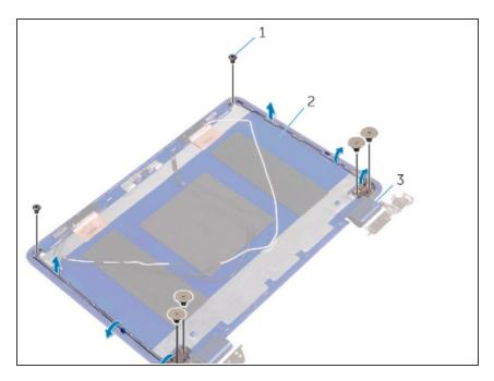
Align the screw holes on the NEW display hinges with the screw holes on the display back-cover and antenna assembly.
