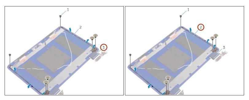
Lift the display hinges off the display back-cover and antenna assembly.
