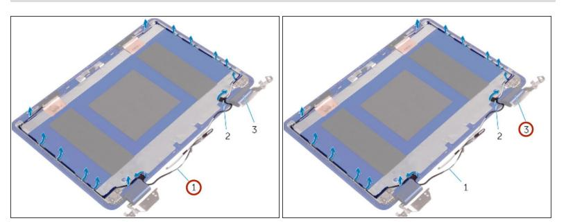
Route the antenna cables through the routing guide on the hinge cover and secure it in place.
