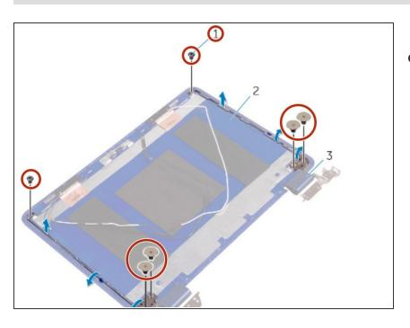
Remove the screws that secure the display hinges to the display backcover and antenna assembly.
