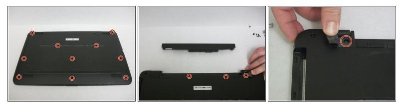
• With the laptop upside down, remove the battery by hand and the twelve 7.0 mm screws that are holding the back case to the front. Use a JIS #0 screwdriver to remove the screws.
