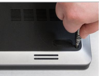
Remove the two 4.5 mm Phillips #0 screws on the access panel door.
