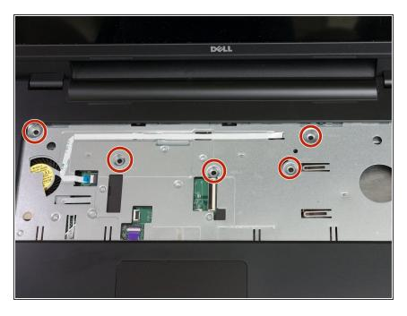
Remove the five 4.5 mm Phillips #0 screws found under the keyboard.
