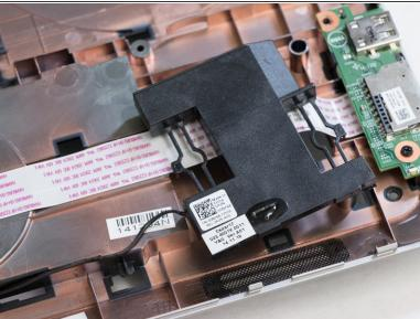
• Using the plastic opening tool, gently remove the second speaker.
