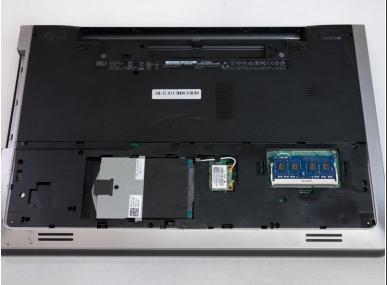
Using a plastic opening tool, pry open the access panel, exposing the disk drive, RAM, and wireless module.
