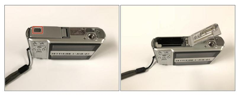
Slide the tab to the left to open the battery cover.
