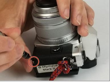
Continuing to use the size PH00 Phillips-head screwdriver, remove the two 3/5 inch screws revealed after removing the bottom plate of the camera.
