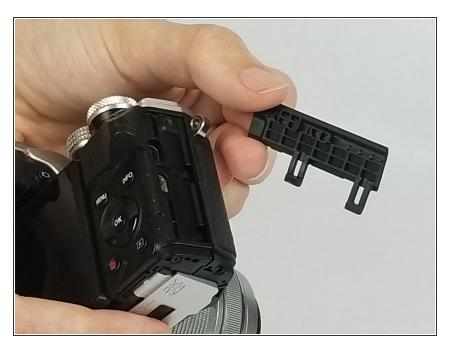
Proper removal of all 11 screws listed in the steps above from the camera gives the camera the ability to be opened slightly and allows for the door to be lifted off of the hooks holding it in place within the camera.
