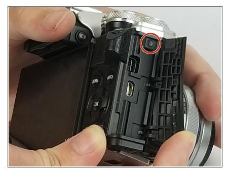
Open the HDMI connector door and continue to use the PH00 Phillipshead screwdriver to remove the 3/10 inch screw located underneath the door.
