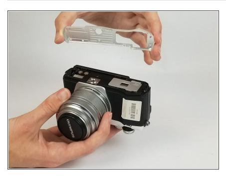
After removing all of the screws, remove the bottom plate from the camera to continue.
