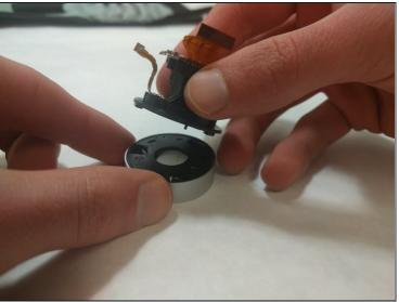
• Remove the three PH000 3.55mm screws that connect the end cap that holds the privacy shutter to the rest of the camera enclosure. Once the screw are removed, you can pull them apart.
