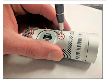
Remove two 3.55 mm screws that hold the body to the ball and socket joint using the PH000 screwhead.
