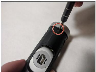
• Unscrew the 3 (3.55 mm) screws surrounding the black casing near the camera-lens.
