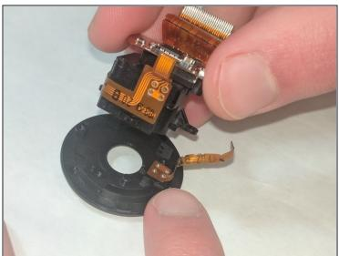
• Unscrew the three PH000 3.55mm screws from the connecting plate and the camera enclosure. Pull apart when all screws are removed.
