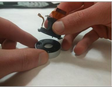
Remove the three PH000 3.55mm screws that connect the end cap that holds the privacy shutter to the rest of the camera enclosure. Once the screw are removed, you can pull them apart.
