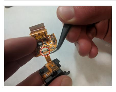
Pull the pin tab from the base of the circuit board to separate the camera module and the lens enclosure.
