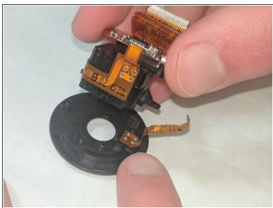
Unscrew the three PH000 3.55mm screws from the connecting plate and the camera enclosure.
