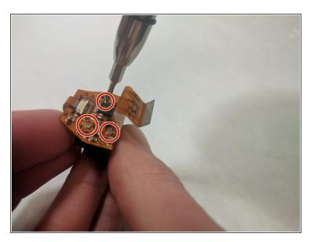
Unscrew the three PH000 3.55mm screws securing the Camera module circuit board and lens enclosure.
