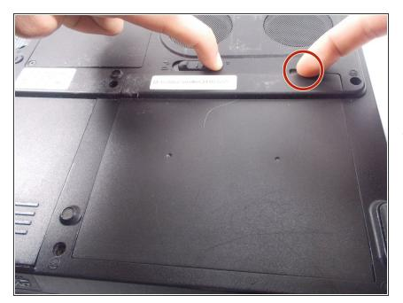
Place your left hand on the locking mechanism and slide it all the way to the left. This will move it into the unlocked position. While holding the mechanism in the unlocked position place another finger in the cavity to the right of the locking mechanism.
